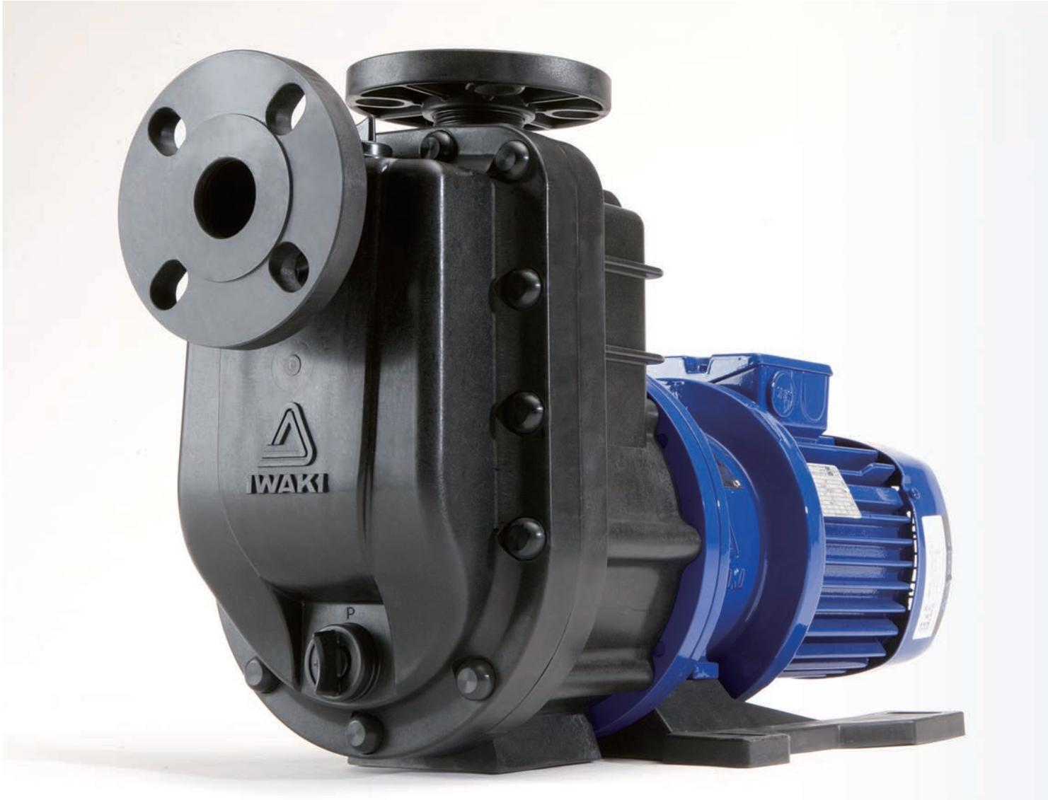
The SMX is a horizontal self-priming magnetic drive pump made from reinforced plastic. Our original self-radiation structure (Patented) enhances resistance to dry running, cavitation, and closed-discharge operation. In addition, the use of standard motors extends the range of application.
